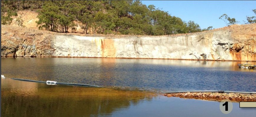
Pit prior to treatment containing 56 megalitres of pH 2.9 acid mine water containing a range of contaminants
