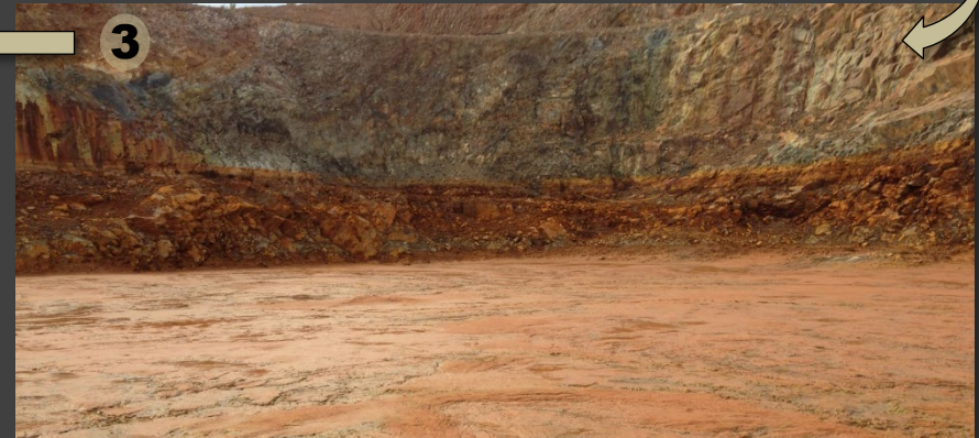
Dewatered pit with hydrotalcite residue "ore" grading 8% Cu and 4% Zn (on dry mass basis)
