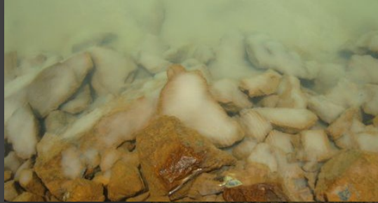
Hydrotalcite precipitate after treatment
